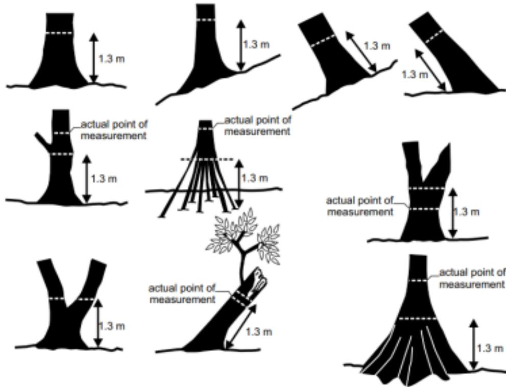
**Figure 2:** Examples of where to measure DBH on a tree that is leaning, on a slope, has multiple stems etc.
